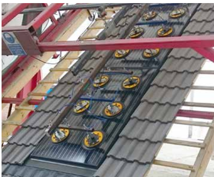
Marley SolarTile® (a Clearline Fusion product) achieved the highest possible wind resistance during testing for MCS012
